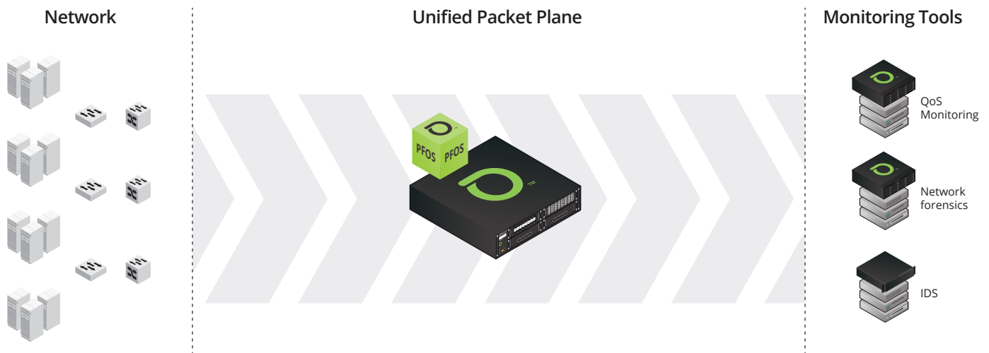
Figure 1: The NETSCOUT unified packet plane powered by PFOS (Packet Flow Operating System) logically separates the network from the monitoring systems.
