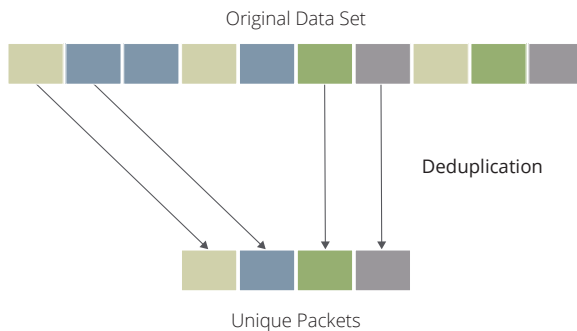
Figure 1: Unique packets are retained as shown, while duplicates are discarded before reaching the tools.
