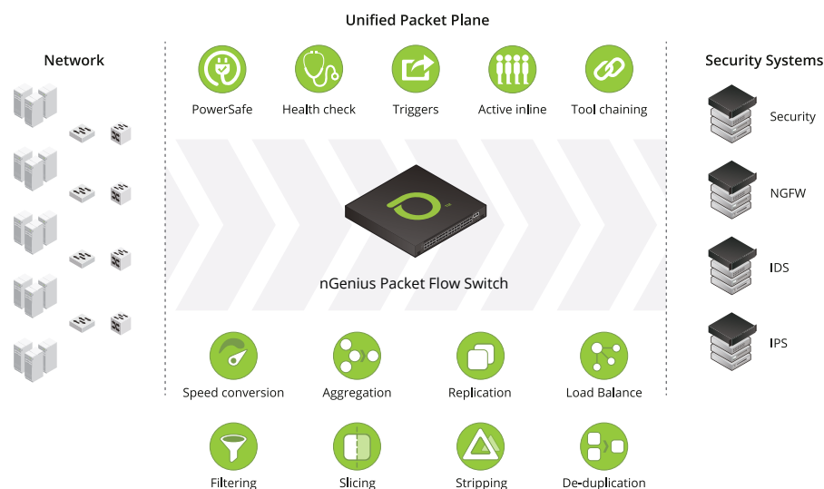
Figure 1: Packet flow systems provide the foundation for a scalable monitoring architecture needed for security and service assurance.
